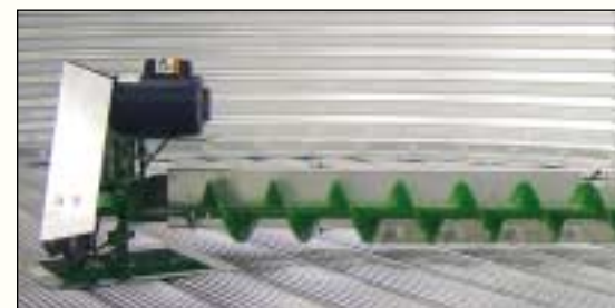
Sukup Tube and Well System with Carry-in Sweep
